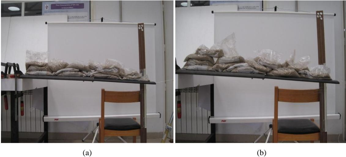
Figure 6: Variable-span wing loaded at: (a) 3.5G – 10.5kgf; and (b) 4.5G – 13.5kgf.
