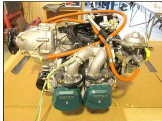
The Rotax 912 ULS power-plant assembly, rated at 100 hp (75 kW) being prepared at MBAS, Whitianga
