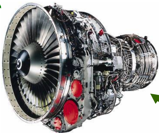
CF6 Aero Engine (core of LM2500 engine)
